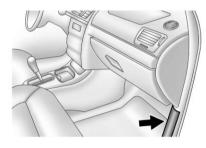
The fuse block is on the passenger side of the vehicle in the carpet molding. Remove the fuse block door to access the fuses.
